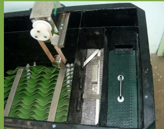
Tramp Oil Separation – Carbon Pre filter
